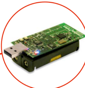
TelosB sensor node platform IEEE 802.15.4 compliant, TI MSP430 microcontroller, 10 kB RAM, 1MB external memory
